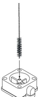
A technical drawing of a membrane cover with a brush being used to clean its top surface. An arrow points from the brush to the cover.            | <p>5. Nettoyer le couvercle de membrane à l'aide d'une brosse de nettoyage Ø max. = 1,5 mm (0,05").</p>                    |
