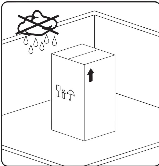
To store the device, place it in its original packaging and store it in an enclosed, dry and frost-free room. Ensure that the storage temperature does not exceed the limits specified on the type plate.
