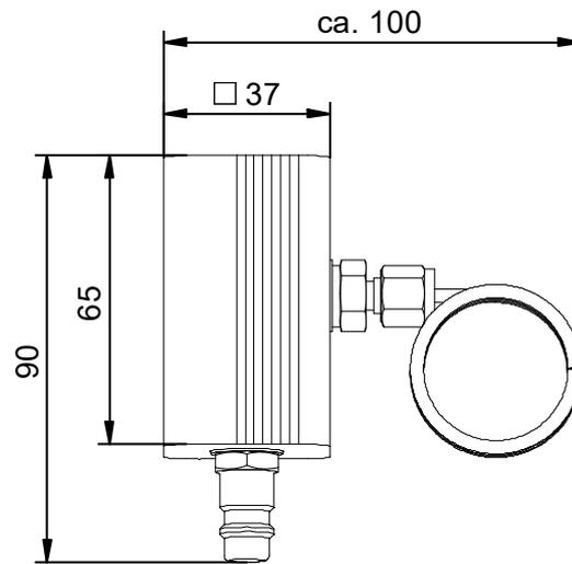
Dimensions measuring chamber with a purge-air controller
