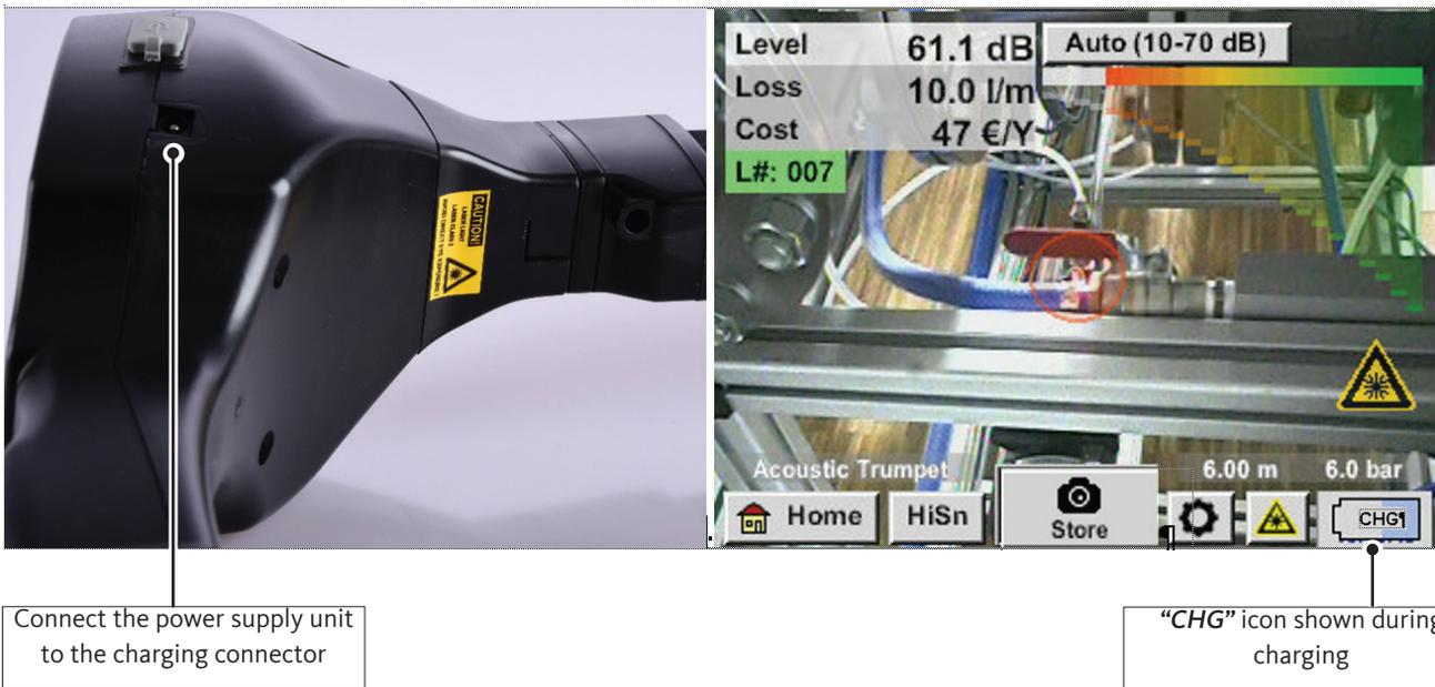
The **METPOINT® CID** will check the battery's state of charge and will start charging it automatically if necessary.
