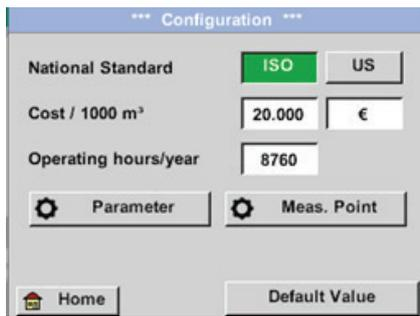
The configuration settings can be used to select the system of units you want and enter the parameters needed in order to calculate annual leakage costs.
