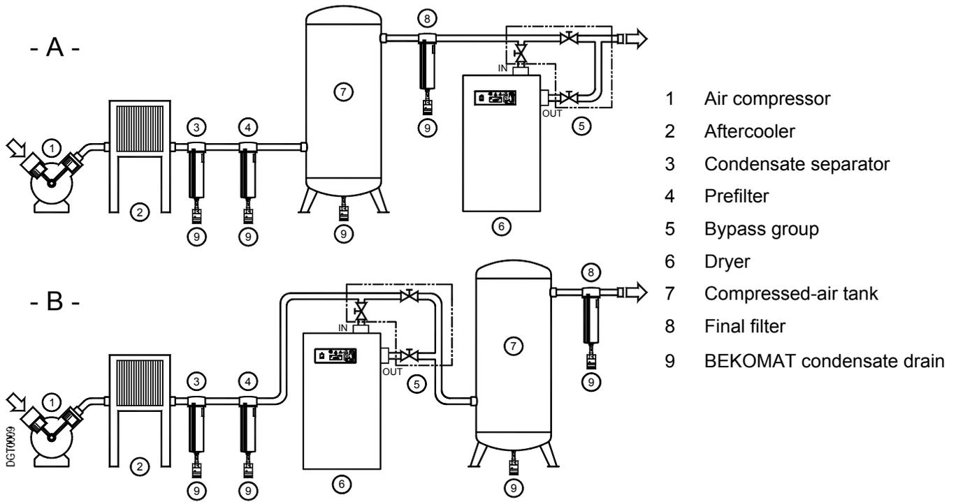
Installation **type A** is recommended when the total consumption corresponds to the throughput rate of the compressor.
