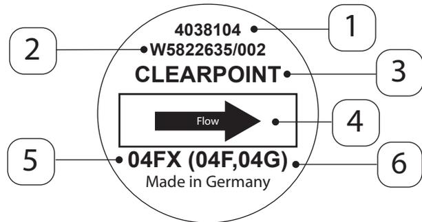
Adhesive filter element label - View filter element base
