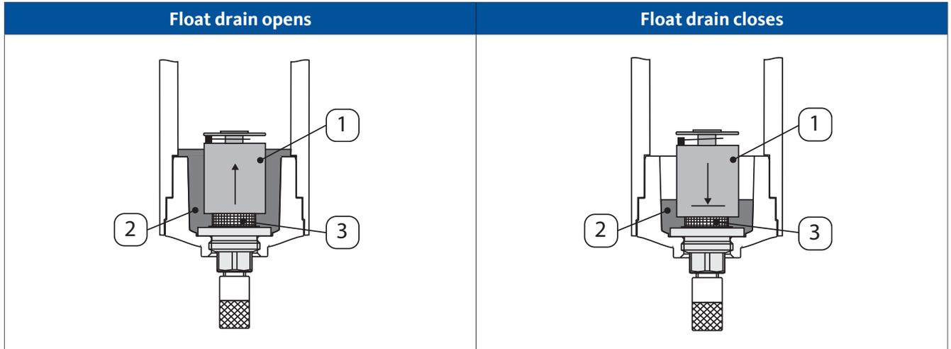
Both types of float drain are delivered with the position "Automatic discharge" from the factory. The knurled screw is screwed downwards as far as it will go.
