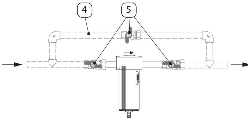
1. Apply sealing material e.g. PTFE-tape (EN 837-2) to the pipe ends.
