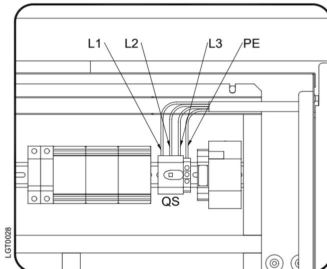
A residual-current device (RCD) with  $I_{\Delta n}=0.03A$  is suggested. The cross-section of the power supply cables must correspond to the consumption of the chiller. In this respect, the ambient temperature, the cable laying conditions, the length of the cables and the requirements of the local electricity supplier need to be considered.
