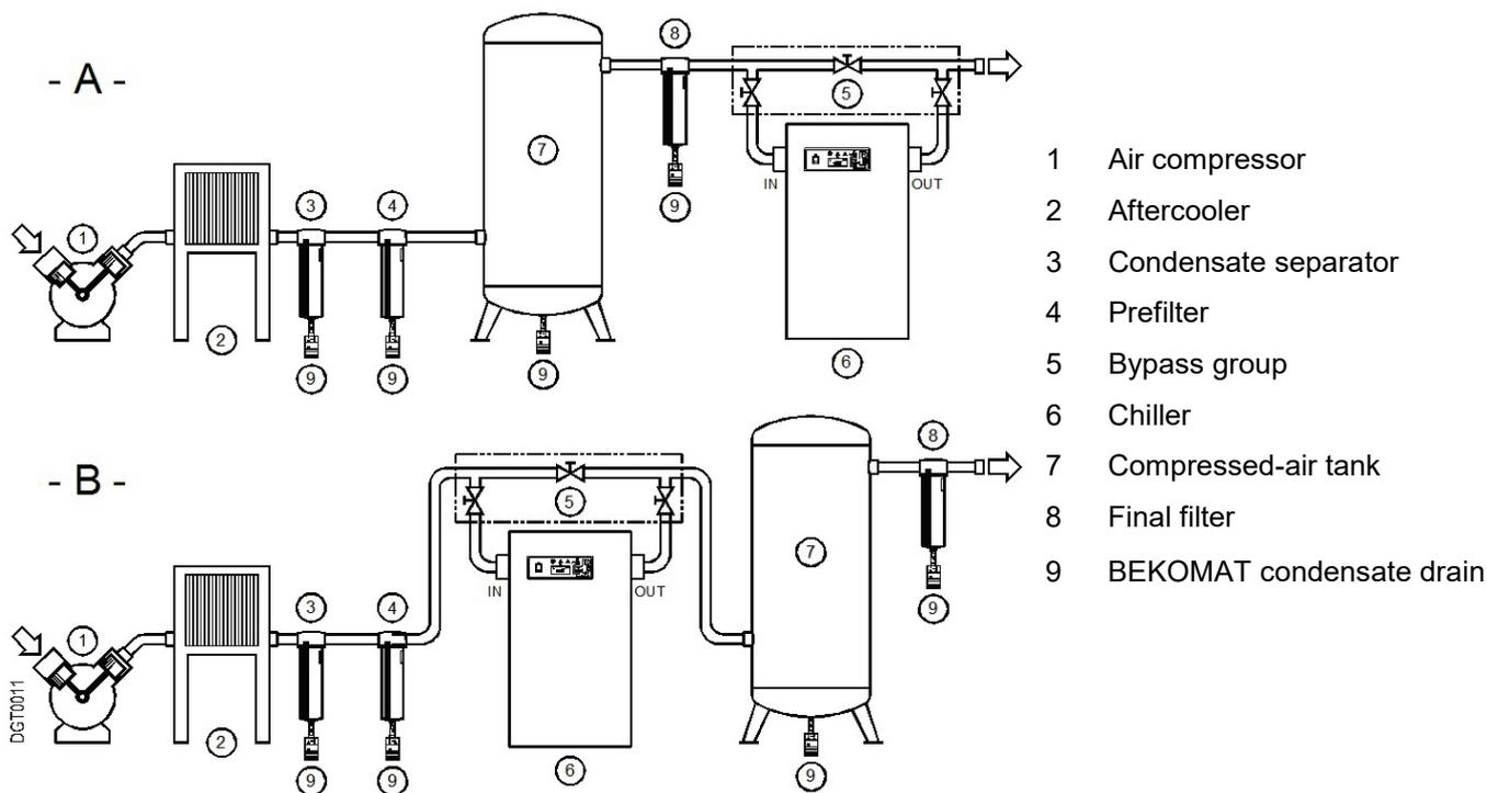
Installation **type A** straight upstream of the application is recommended.
