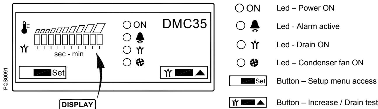
The DMC35 displays DewPoint temperature, controls the condenser fan activation, controls the timed drainer and keep record of the total hours of operation of the dryer.
