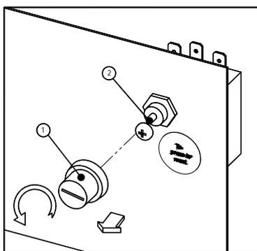
To ensure the operational safety and the soundness of the chiller, a safety temperature switch (TS) is installed at the refrigeration cycle. In the event that the pressure gas temperature is too high, the sensor of the temperature switch will stop the refrigerating compressor to prevent the pressure gas temperature getting too high.
