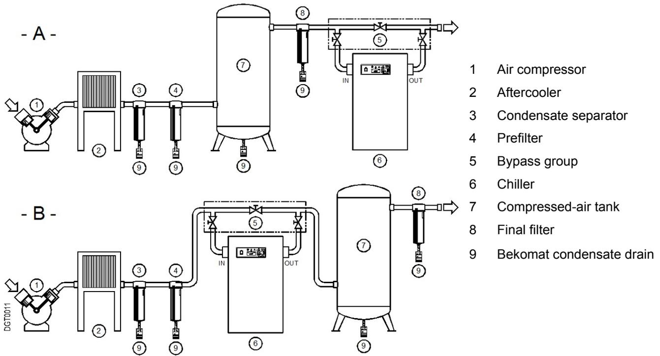
Installation **type A** straight upstream of the application is recommended.
