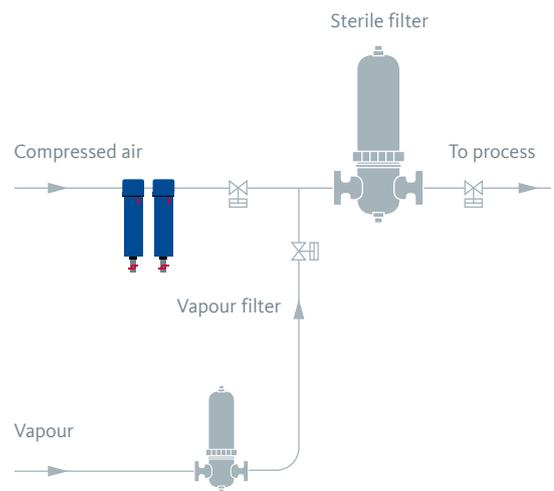
Vapour sterilisation in direct flow; Flow direction from hot vapour through the sterile filter is identical with the through-flow direction for compressed air.
