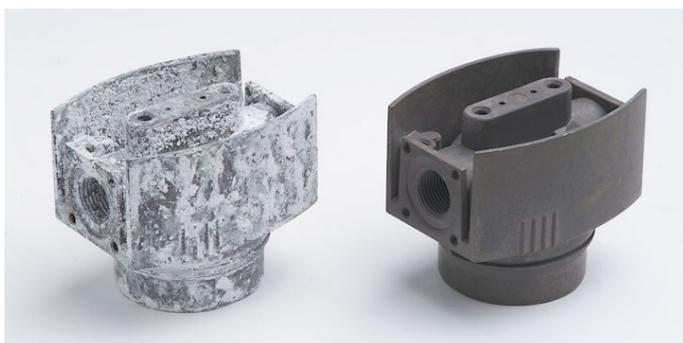
Seawater resistant aluminium optimally protects the streamlined housing against corrosion – exactly like the complete anodising and externally applied additional powder coating. CLEARPOINT® high-pressure filters are therefore also resistant to aggressive condensate.
