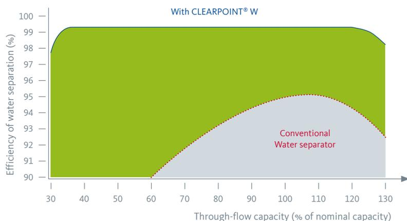
The CLEARPOINT® W with flow-optimised design achieves an efficiency of up to 99% over a wider performance range – for highest possible separation-percentages with lowest costs.
