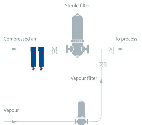
Vapour sterilisation in counter flow: Flow direction from hot vapour through the sterile filter is opposite to the through-flow direction for compressed air.
